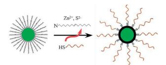
One small step: A facile and robust onestep method for creating stable, watersoluble quantum dot (QD)-biomolecule conjugates is described. DNA molecules can be readily attached to QDs during core-shell synthesis (see picture of DNA functionalization of a CdSe@ZnS coreshell QD).
